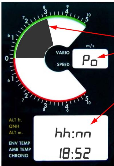
The power On display shows the battery status, and the current time and date
