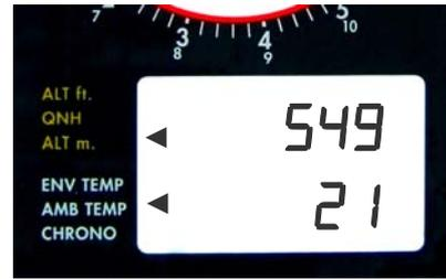
1. Press altimeter key for 4sec. until display is blinking.
