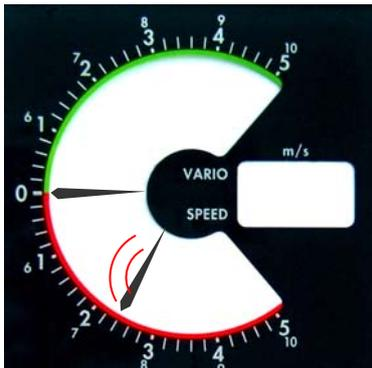
The threshold point is displayed in the analog vario display with a blinking segment.
