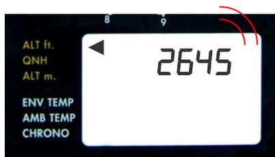
A long press on the yellow key ALTI brings the device to the set mode of the current activated function **Alt. ft**, **QNH** or **Alt. m**
