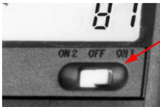
After switching ON, the device performs a self test and displays for 10 seconds the the battery condition of the activated battery in the variometer screen.
