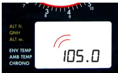
By pressing the **TEMP ALARM** key for 4 sec., the temperature alarm function is activated. (Display is blinking)
