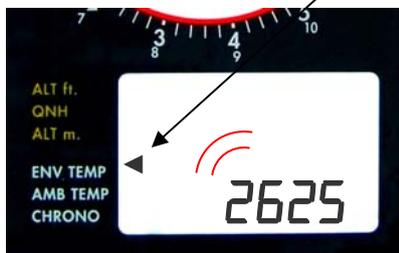
Select in the lower Display by pressing the **ENV TEMP** Key the ENV TEMP Function. (The arrow indicator points to ENV TEMP).
